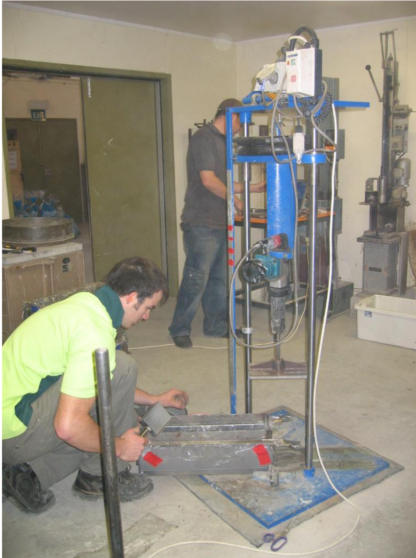
Figure 15 – Compaction frame with vibrating hammer and foot for beam manufacture.
