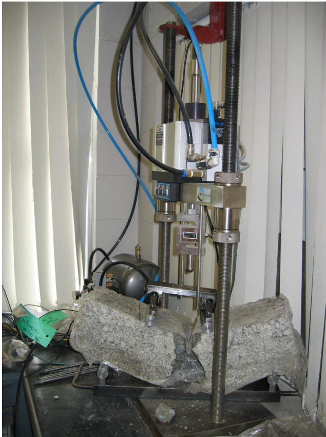
Figure 19 – Result after breakage or fatigue test.
