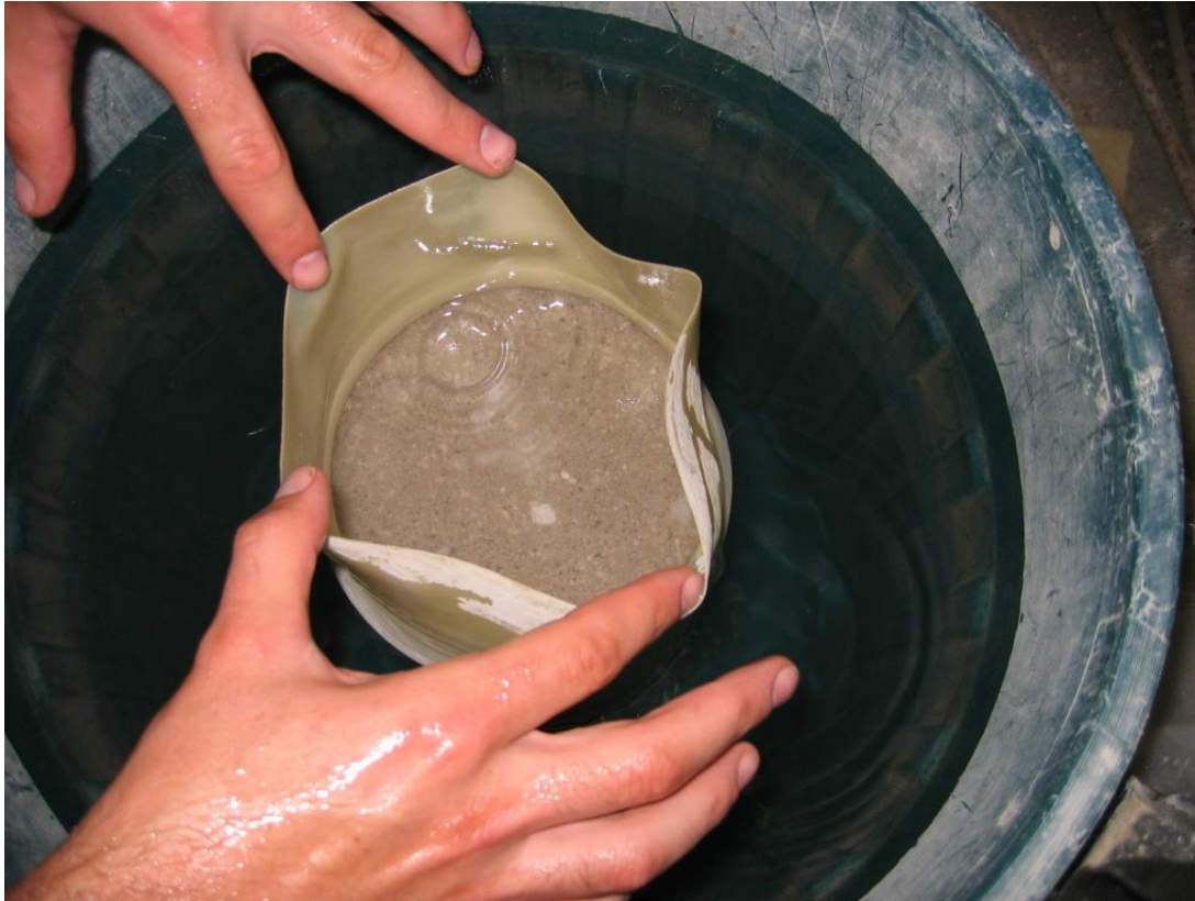
Figure 3 – Soaking sample for saturated undrained RLT test.
