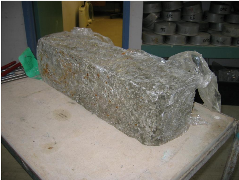
Figure 17 – Compacted and cured beam ready for testing.
