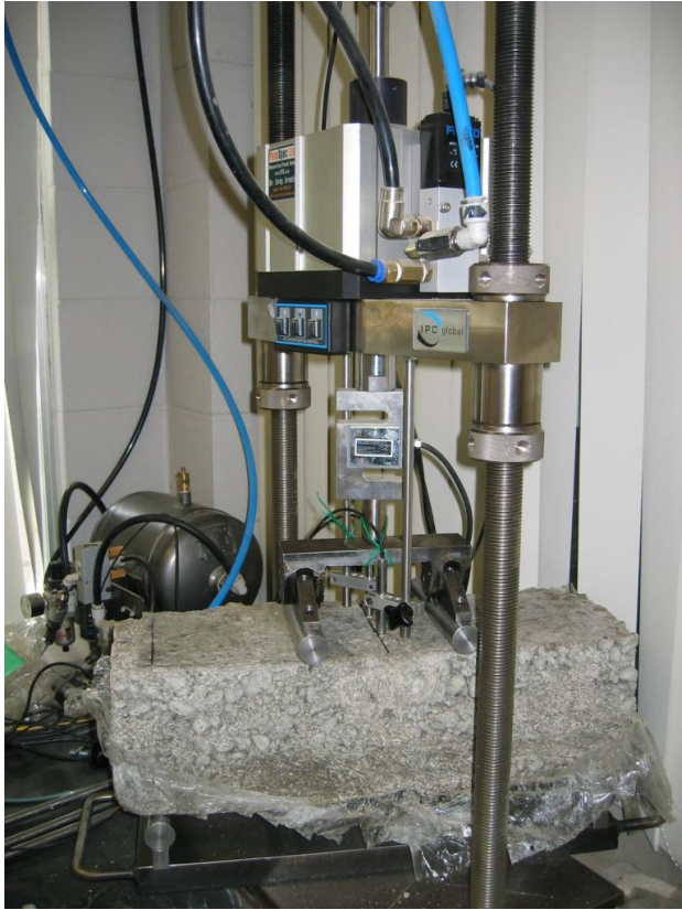
Figure 18– Test setup for measuring flexural beam properties.
