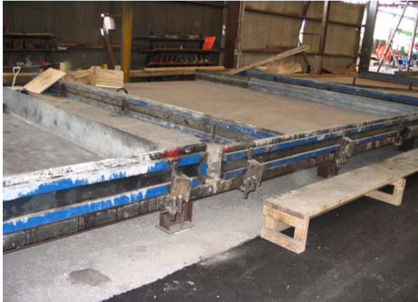
Flat Beds for Wingwalls & Fenderwalls
