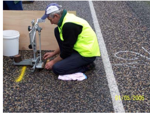
Figure 6. British Pendulum test on a 85/15 blend
