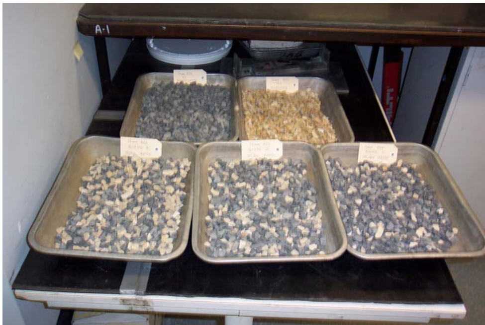
Figure 4. Blended products, basalt (control) and volcanic tuff.
