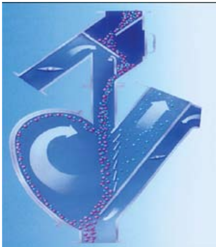
Operating principle of the AC27/AC30 gravitational inertial classifier.
